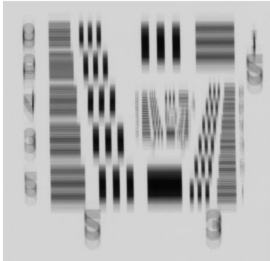
Figure 19: Image with incorrect scan direction
