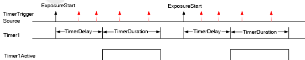
Figure 8-66 The relationship between Timer1Active and the ExposureStart signal
