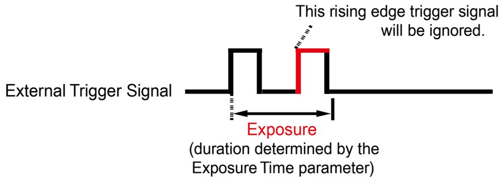
Figure 4-5 Trigger Overlapped with Time Exposure Mode
