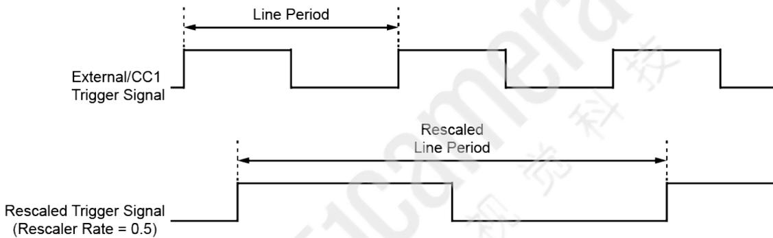
Figure 4-3 Trigger Ratio = 0.5
