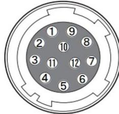
Figure 3-4 Pin Assignment of the Power Input Receptacle
