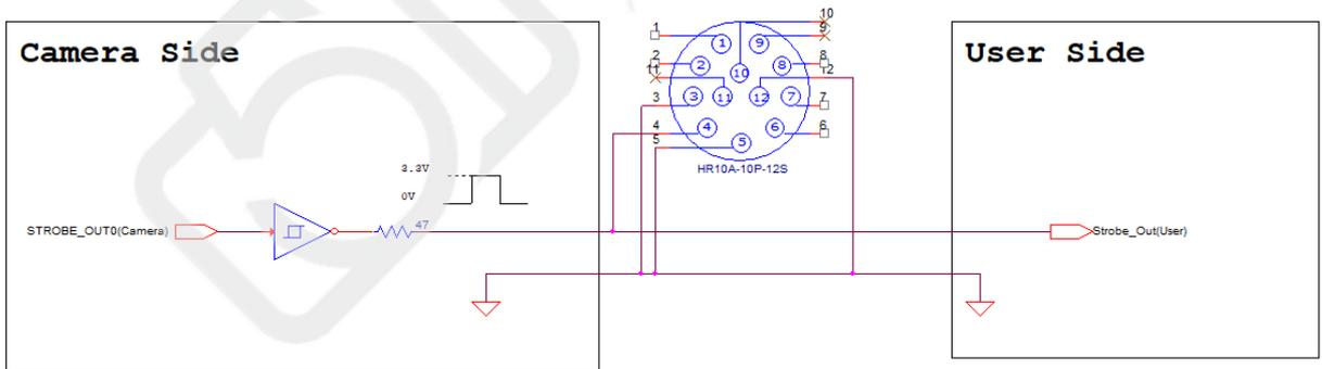
Figure 3-2 Output Schematic
