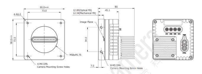
• VTS-9K5X2 UV Camera with two additional heatsinks (Heatsink Size: 87mm x 39.5mm x 78.5mm)
