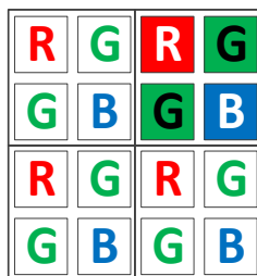
Figure 8-48 Horizontal and vertical color Binning by 2x2
