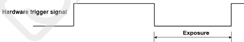
Figure 8-29 The sequence diagram in falling edge trigger of TriggerWidth exposure mode
