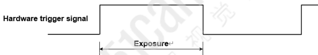
Figure 8-28 The sequence diagram in rising edge trigger of TriggerWidth exposure mode
