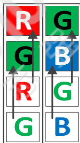
Figure 8-47 Vertical color Binning by 2
