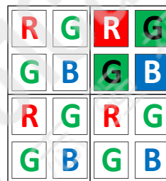
Figure 8-49 Horizontal and vertical color Binning by 2x2
