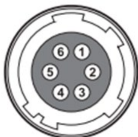
Figure 3-4 Pin Assignments for 6-pin Control I/O Receptacle
