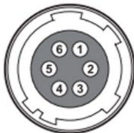
Figure 3-3 Pin Assignments for 6-pin Power Input Receptacle
