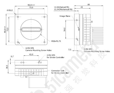
• VTS-9K5X2 (Camera + 2 Additional Heatsinks), Heatsink Size: 87mm x 39.5mm x 78.5mm
