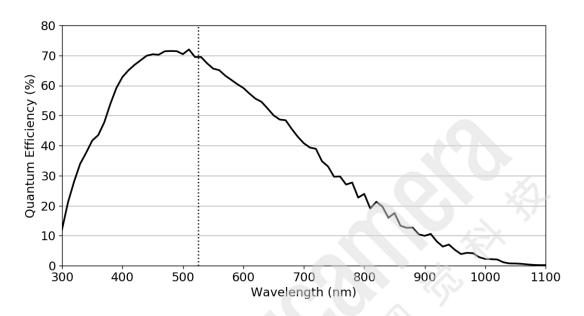
Forge FG-P5G-244S8C Spectral Response Curve
