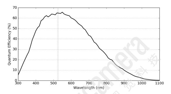
Firefly FFY-U3-04S2C Spectral Response Curve
