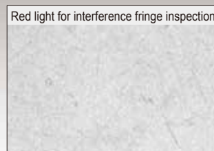
Interference fringes are not visible when there is no coating
