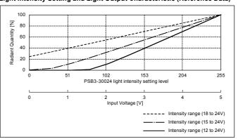
Note: The above data represents actual results for the LNSD-400SW-HU(A) Light Unit. (This data is for reference only.) The graph for the LNSD-400SW(A) Light Unit is the same.
