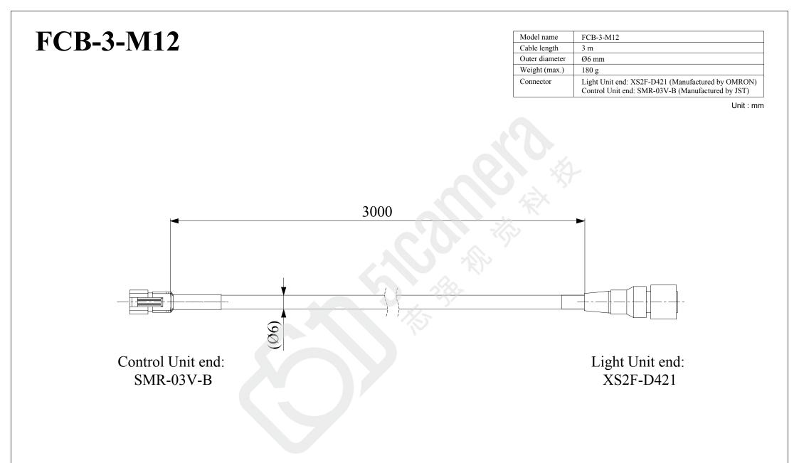
\*The connector on the Control Unit end is not waterproof.
