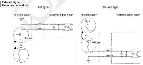
Becomes HIGH when 24 V is applied to input+ and 0 V is applied to input-. Apply a current using the open-collector circuit, high-speed photocoupler, semiconductor relay, and so on. (We recommend 10 mA or less.) The pulse width must be 10 µs or more (Applied voltage 24 V±10%).
