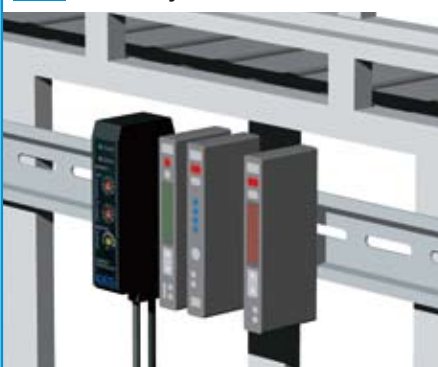
4 Install in available space under assembly lines or below racks.
