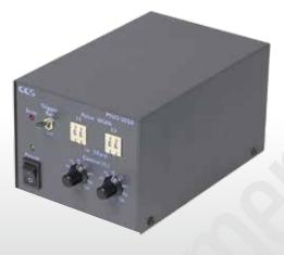
The PTU2 series enables strobe lighting with overdrive. Overdrive refers to brighter than normal emission of light by increasing the voltage and current supplied to the Light Unit.
