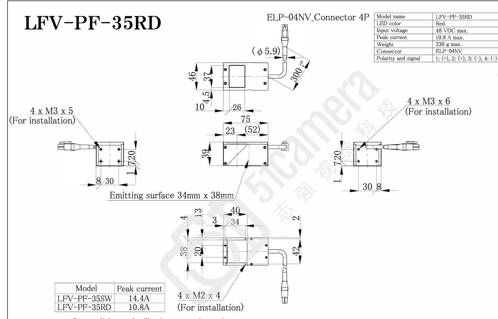
Do not light up the illuminator continuously. This illuminator has some restrictions for light-up condition. Please keep strictly the duty cycle under 1% and pulse width under  $500 \mu$  s.
