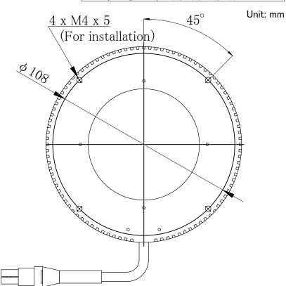
&Do not light up the illuminator continuously. This illuminator has some restrictions for light-up condition. Please keep strictly the duty cycle under 1% and pulse width under 500  $\mu$  s.
