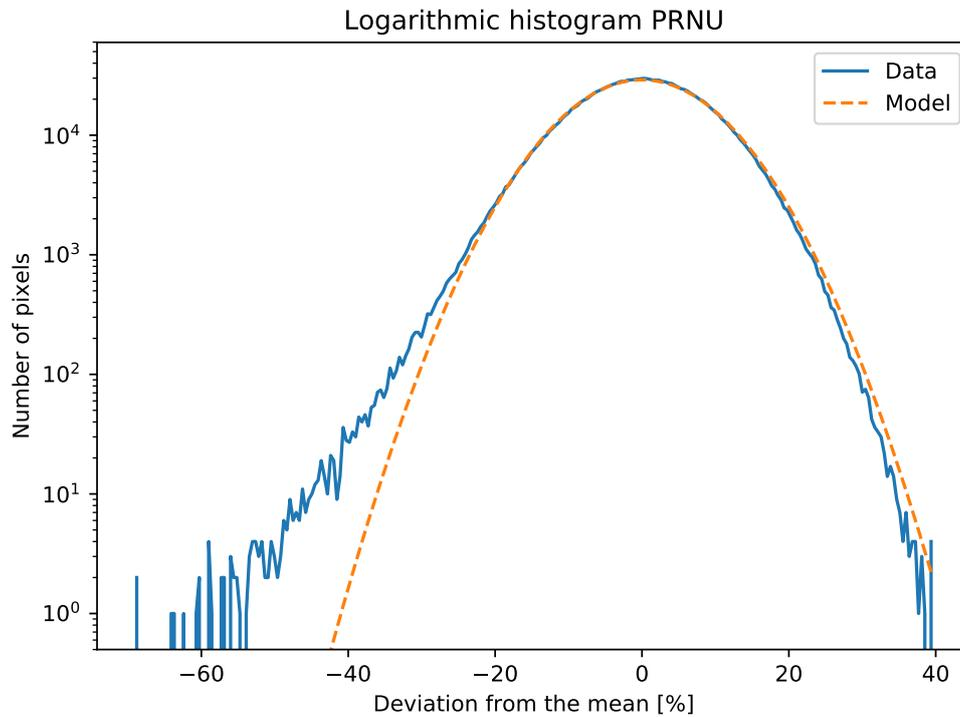
Accumulated logarithmic histograms for dark signal nonuniformity (DSNU) and photoresponse non-uniformity (PRNU) are plotted versus the deviation from the mean gray value of the image. This yields the probability distribution of the absolute deviation from the mean value. Thus it gives the number of pixels that show at least a certain absolute deviation from the mean.
