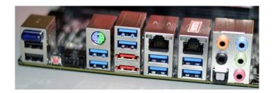
Figure 4. A motherboard with 8 USB 3.0 ports
