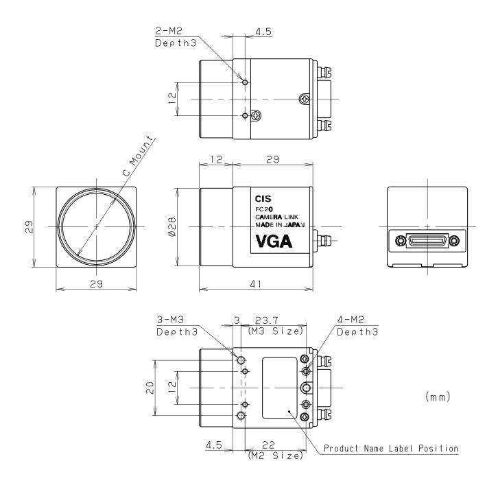
% C Mount screws comply with ANSI/ASME B1.1, 1-32UN(2B)
