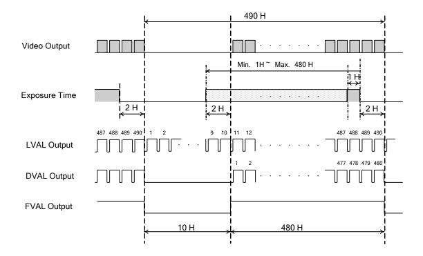
XVideo output signal delays by 2H from Exposure Time.
