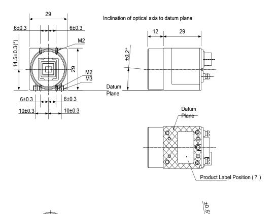
Inclination of effective pixels, Theta,?, to datum plane shall be ??  $\pm 0.5^{\circ}$  The center of effective pixels shall be within f 0.6 to the center of C lens mount
