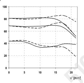
The Modulation Transfer (MTF) as a function of image height (u) and slit orientation (sagittal, tangential) has been measured with white light at spatial frequencies of R=10, 20 and 40 cycles/mm.
