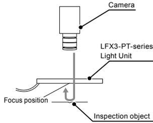
When the ambient light is reflected from the surface of the Light Unit or the surface of the inspection object, the captured image may be affected.
