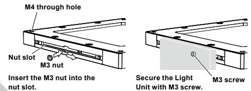
Determine the length of the screws considering the dimensions of the M4 through holes and nut slots. For information on the dimensions of each part, refer to 8. *Dimensions*.
