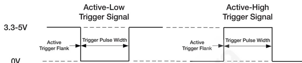
Figure 5.7. Trigger Polarity
